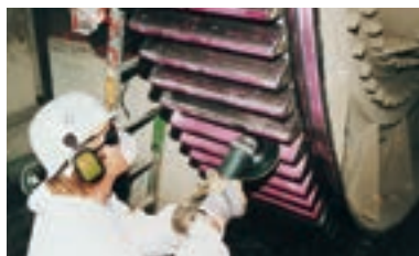
Treatment of the working tooth flanks.
